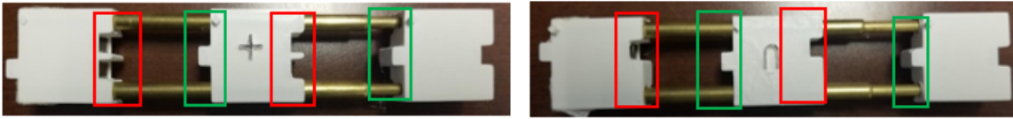
Figure 3: Left: PLUS operator with expandable slots, Right: AND operator with expandable slots. Both: telescoping tubes appear as parallel sets of brass tubing between each block in the expandable elements. Note that neither assembly includes the texture and color for Operator blocks.
