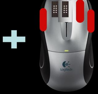
2 Braille pin output3 Pushbutton inputs
